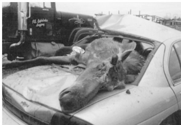
Fig. 4—Significant impact of moose with roof and windshield of vehicle.
